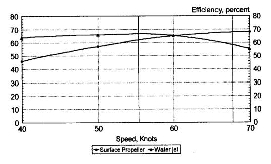
The above plot of the relative efficiencies is similar to the results documented in the paper by Kruppa(3). The net average for the entire operating range is what is important here, 40 - 68 knots. The net efficiencies are good.
