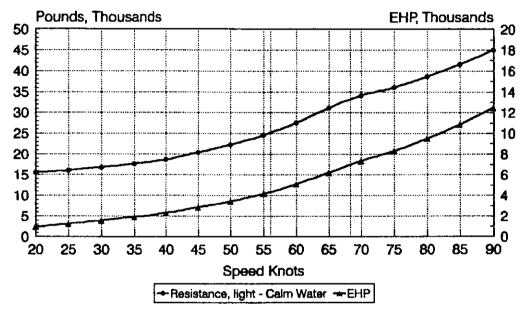
At seatrials in calm seas in the light condition the speeds were documented at 68 knots with all systems running and 56 knots with only water jets with diesels. To keep this in a proper perspective these calculations are only to be used as an estimate.
